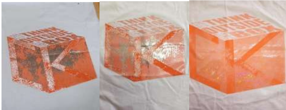
Figure 5. Repairing experiment used silver and clear rainbow foils taking advantage of the “sticky-flaw” of the rejected print to make it adhere foil layer by amending the normal foil pressing conditions (Source: Author)
