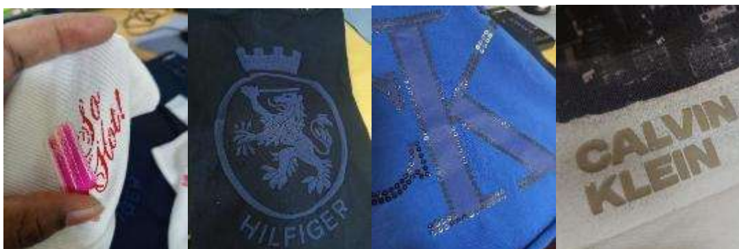
Figure 4. Examples of defective screen-printed textile samples rejected during quality inspection (Source: Author)
