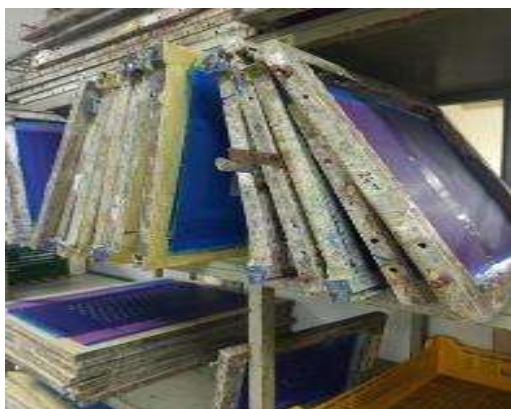
Figure 6. Stored screen-printing frames from previous production batches (Source: Author)
