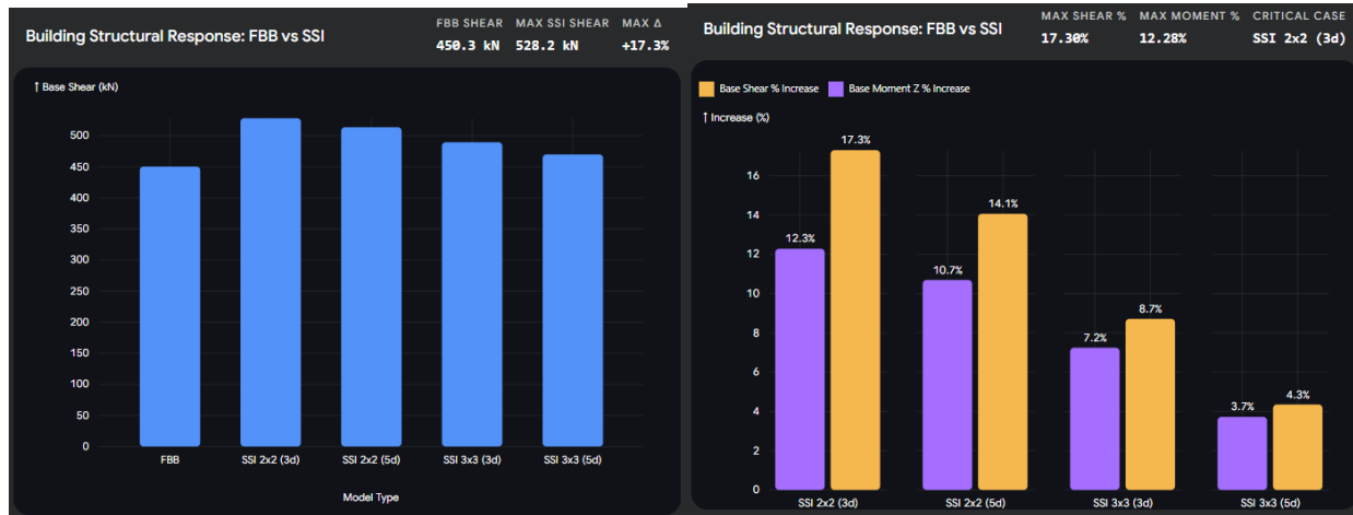
Figure 3: Representation of the base shear force comparison across multiple foundation configurations, demonstrating the 17.30 percent increase in demand for soft soil environments
