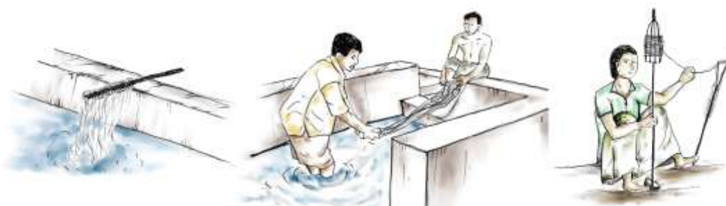
Fig. 13. Washing the yarn multiple times, drying and brushing or smoothing them (from left) (Source: Author)
