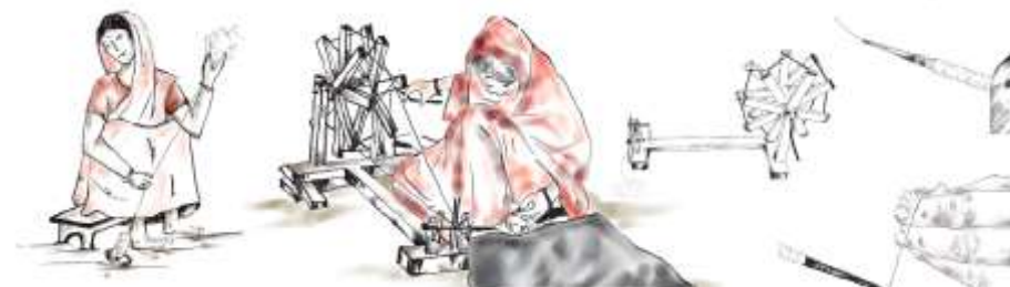
Fig. 10. Hand spindling yarn, hand spinning wheel, Natai or warping the yarn (from left) (Source: Author)
