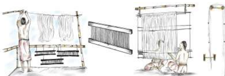
Fig. 16. Making Sana or reeds with bamboo sticks, drying the Sana and yarn, Sana Badha (Source: Author)
