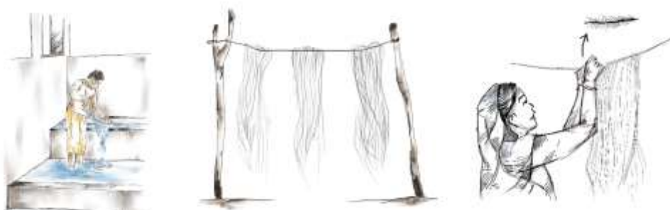
Fig. 13. Washing the yarn multiple times, drying and brushing or smoothing them (from left) (Source: Author)
